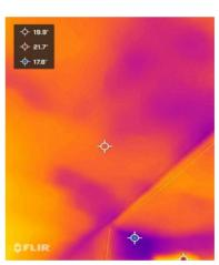
The loft area over the outrigger has recently had the insulation topped up to 300mm. It is important that the insulation covers all areas, including the difficult to reach areas beyond the purlin timber. It is also important to maintain adequate ventilation to the loft space. Loft hatches should be insulated and draught proofed.
